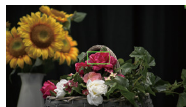
Focus icon turns green when accurate focus is achieved manually.
